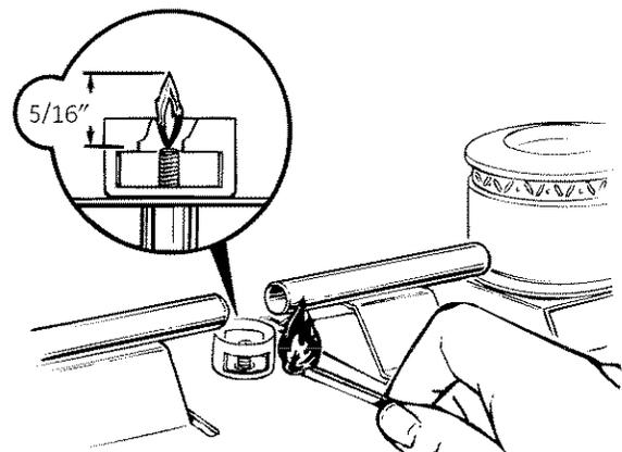
**NOTE:** Do not leave standing pilot lit in a newly constructed or remodeled home or apartment that will be unoccupied for more than a month.
