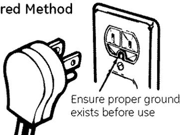
The power cord of this appliance is equipped with a 3-prong (grounding) plug which mates with a standard 3-prong grounding wall receptacle to minimize the possibility of electric shock hazard from this appliance.
