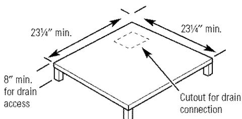
2. Place the platform in the utility closet with the following clearance between it and the interior surface of the walls/door/panel:
