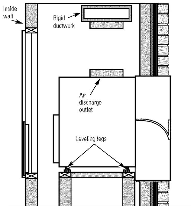
3. Using field-supplied screws, bolt the case to the platform.
