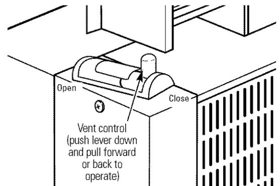
**Energy Tip:** Keep the vent control in the **CLOSE** position. The room air will be filtered and circulated.
