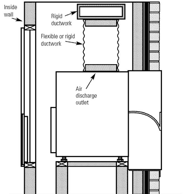
2. Secure the top duct to the unit by turning the four case top duct adjusting screws until they are tight. Use a field supplied clamp to lock the top duct to the case.
