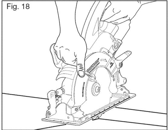
4. You **must** release the lower blade guard lever as the blade enters the material.
