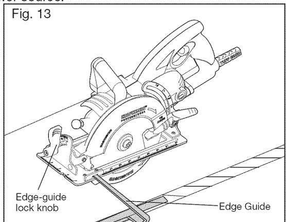
When using the edge guide, position the face of the edge guide firmly against the edge of the workpiece. This will help to make a true cut without binding the blade. The edge of the workpiece must be straight for the cut to be straight. Use caution to prevent the blade from binding in the cut.
