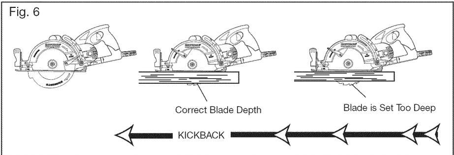
9. **Use extra caution** when making a “Pocket Cut” into existing walls or other blind areas. The protruding blade may cut objects that can cause Kickback.
