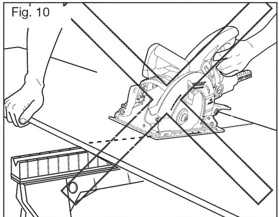
**Never** place the saw on the part of the workpiece that will fall off when the cut is made.
