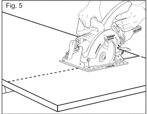
2. If the blade is binding or when you are interrupting a cut for any reason, **always** release the trigger and hold the saw motionless in the material until the blade comes to a complete stop. **Never** attempt to remove the saw from the workpiece or pull the saw backward while the blade is in motion, or kickback may occur. Check and take corrective action to eliminate the cause of blade binding.
