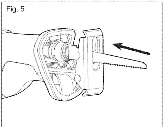
**NOTE:** The blade may be installed with the teeth pointing up or down, according to the needs of the cutting operation.
