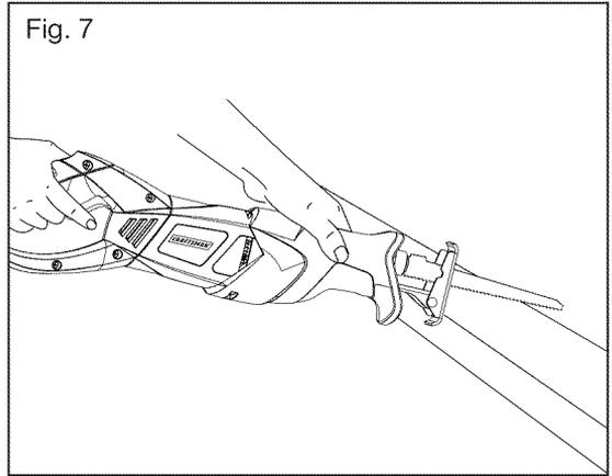
**NOTE:** Cutting speeds should vary with the workpiece. Hard materials, such as metals, require lower speeds; for softer materials use higher speeds.
