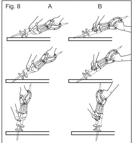
**Note:** To make plunge cutting easier, use a heavy gauge blade and install the blade with the teeth facing upward as show in colum B.
