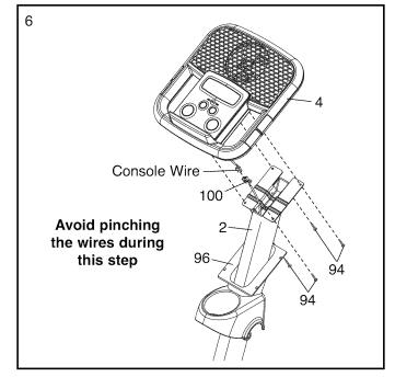
Slide the Console Cover (96) (see the drawing in step 6) upward to the Console (4). Attach the Console Cover with four M4 x 16mm Screws (84).
