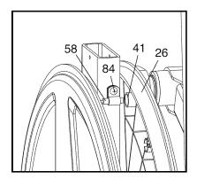
Reed Switch slightly closer to or away from the Magnet, and then retighten the Screw. Rock the Left Pedal Disc forward and backward just enough that the Magnet passes the Reed Switch repeatedly. Repeat
