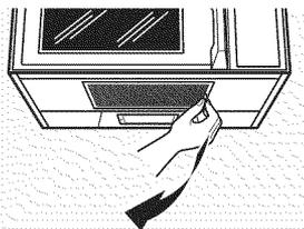
**To remove**, slide it to the side using the tab. Pull it down and out.
