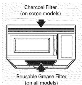
The vent fan has a metal reusable grease filter.
