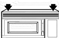
Remove 2 grille screws to remove the grille.
