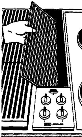
**Filter:** Turn off ventilation system before removing. Turn filter retainer clip to remove filter. The filter is a permanent type and should be cleaned when soiled. Clean in sink with warm water and liquid dishwashing detergent or in dishwasher.
