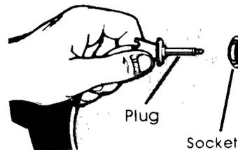
2. Place food in the oven and plug the probe into the socket on the oven wall. The Probe Signal Light will come on.
