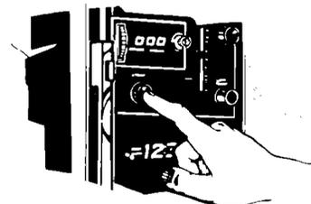
6. Push the START Button. When the probe senses the cooking temperature, a buzzer sounds, and the oven turns off.
