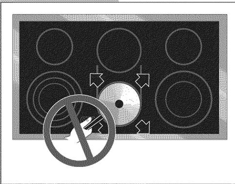
Sliding aluminum or copper clad bottom pans on the cooktop can cause metal markings on the cooktop surface. These marks should be removed **immediately** after the cooktop has cooled using the cooktop cleaning cream. Metal marks can become permanent if not removed prior to future use.
