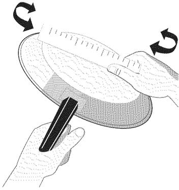
Cookware should have flat bottoms that make good contact with the entire surface heating element. Check for flatness by rotating a ruler across the bottom of cookware. Be sure to follow the recommendations for using cookware has shown in figure aside.
