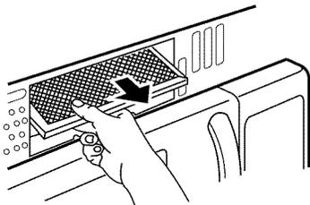
5. Slide a new charcoal filter into place. The filter should rest at the angle shown.
