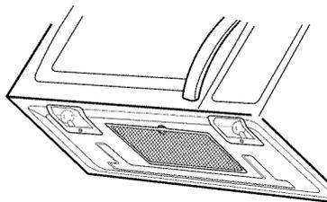
2. Remove the bulb cover mounting screws.
