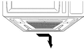
2. Wash in dishwasher or soak grease filter in hot water and a mild detergent. Rinse well and shake to dry. **Do not use ammonia or place in a dishwasher. The aluminum will darken filter.**
