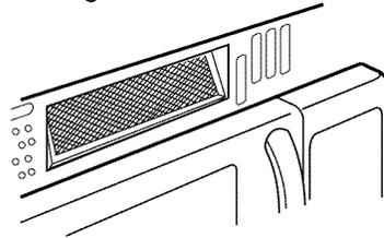
6. Slide the bottom of the grille into place. Push the top until it snaps into place. Replace the mounting screws. Turn the power back on at the main power supply and set the clock.
