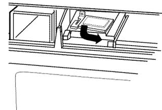
6. Replace bulb with a 30 or 40 watt appliance bulb.
