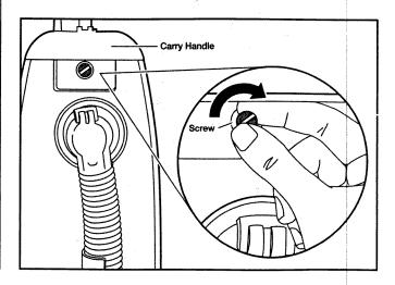
Using a screwdriver, tighten the screw.
