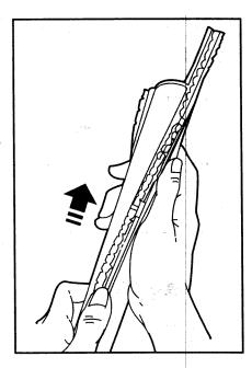
in warm water for a few minutes before sliding them into the slots. Do not use oil. Dry thoroughly before reinstalling.
