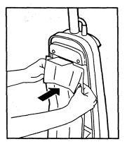
Position the bag cover so its positioning tab fits into the body positioning tab slot.
