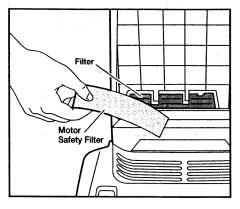
Check the filter located below the foam filter.
