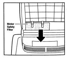
If the foam Motor Safety Filter located at the base of the bag cavity is dirty, remove it by pulling forward.
