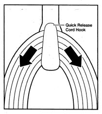
1. Turn the quick release cord hook to either side and down to release the power cord.
