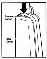
Pull the bag cover forward. Remove and lay aside.
