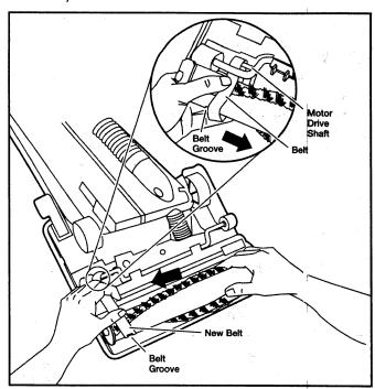
Loop the new belt on the motor drive shaft.
