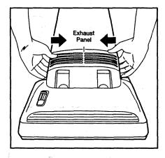
Grasp the air exhaust panel with a hand on each side, press inward and pull the panel forward.
