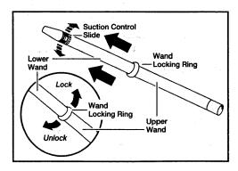
Attach the wand to the hose by inserting and twisting slightly.
