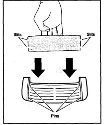
Replace the dry foam filter, carefully positioning it so the slits fit around the four raised pins.
