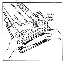
Position hands on the brush assembly. If the belt is still attached to the roller there will be tension on the brush assembly. If belt is not broken remove it from the motor drive shaft before lifting the brush assembly.
