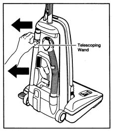
Remove the crevice tool from its storage position in the wand. Turn the locking ring to the UNLOCK position.
