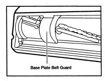
When brushes are worn to the level of the base plate belt guard or when the back-up beater bar is chipped or gouged, replace the brushes.
