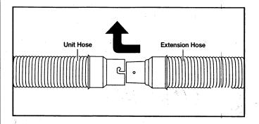
The extension hose has two tabs on the end that can be pushed into the slots and twisted to attach the two hoses together.
