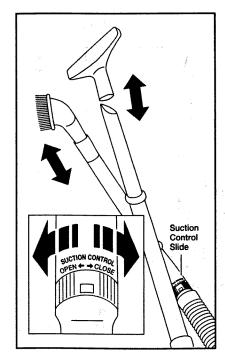
When using the dusting brush or the upholstery tool, they may be attached directly to the wand or placed on the end of the crevice tool.
