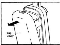
Pull the bag cover forward. Remove and lay aside.
