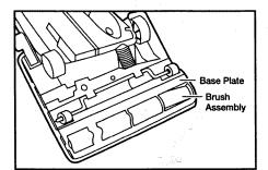
Turn the unit over so the brush assembly and base plate are facing upward.
