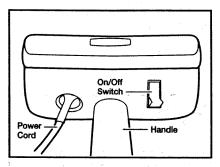
To start the vacuum cleaner, put the switch on the top of the body in the ON position. To stop the vacuum cleaner, put the switch in the OFF position.
