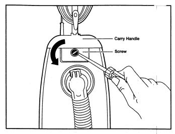
Remove the screw located just below the carry handle on the back side of the vacuum.
