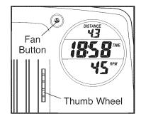
If the fan is turned on but the pedals are not moved for thirty seconds, the fan will automatically turn off.
