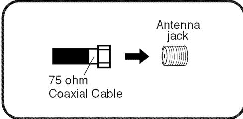
For basic Cable TV service not requiring a Converter/Descrambler box, connect the 75 ohm Coaxial Cable directly to the Antenna Jack on the back of the TV.
