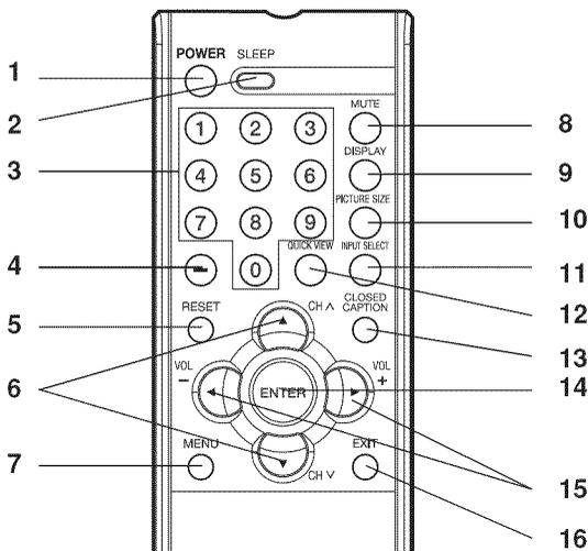
1. **POWER Button** - Used to turn the power on/off to the LCD TV.
