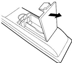
2. Install two “AA” batteries (supplied).
