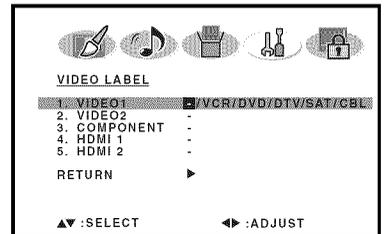
**3** Press ◀ or ▶ to select the desired label for that input source.
