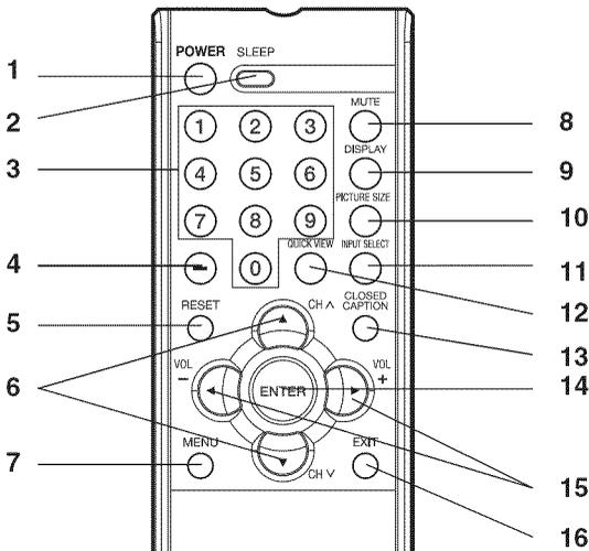
1. **POWER Button** - Used to turn the LCD TV.
