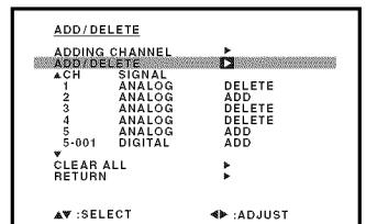
4 Select the desired channel to be memorized or deleted using ▲ or ▼. Press ◀ or ▶ to select "ADD" or "DELETE", whichever function you want to perform.
