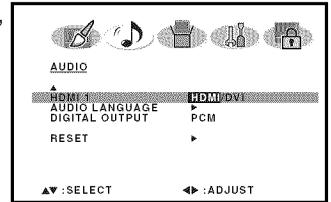
**HDMI:** When you connect the HDMI device to the TV, select this setting.
