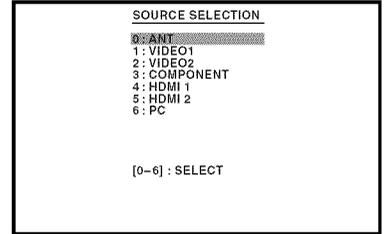
Pressing **INPUT SELECT** on the remote control displays the current signal source. To change the video input source, press **INPUT SELECT** again or **0-6**.
