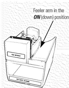
When the refrigerator has been connected to the water supply, move the feeler arm to the **ON** (down) position.
