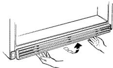
Remove the base grille by pulling out at the bottom.
