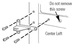
Place the center hinge bracket over the holes at the center left side of the cabinet. Insert and tighten the three long screws.
