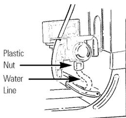
At the front of the refrigerator, unsnap the hinge cover at the bottom of the fresh food door. Remove the base grille and unclip the water line from the hinge area and from behind the base channel. Pull the tubing through to the front of the refrigerator.
