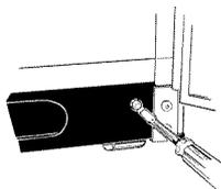
Turn the two front roller adjusting screws clockwise to raise the refrigerator, counter-clockwise to lower it.
