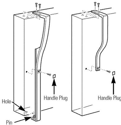
*Models with long handles have a pin that fits into a hole at the bottom of the door.*
