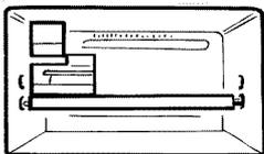
For models with an icemaker, the shelf must be placed in the lower position.
