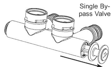
Note: Stem may be installed in either direction. The end with writing should be pulled out for service position.
