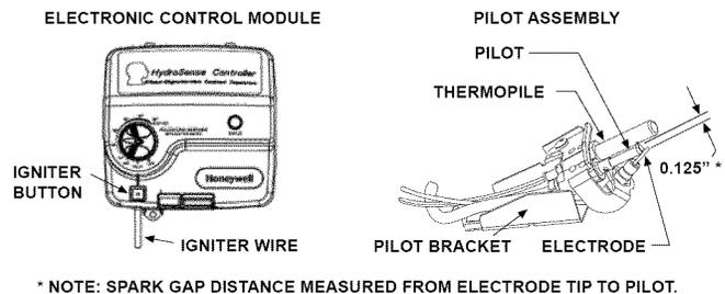
\* **NOTE:** SPARK GAP DISTANCE MEASURED FROM ELECTRODE TIP TO PILOT.
