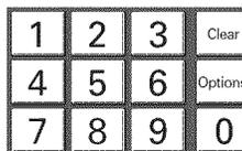
6 Touch the numeric keys in the display (Touch **1**, **2**, and **0**, **0**) and then touch **Options** for selecting **am** or **pm**. The oven door will lock and the display will show the start time. If the oven clock is set to 24 hours display, **Options** will not be able to function for selecting **am** or **pm**.
