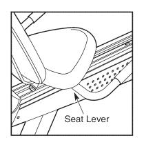
forward or backward, and then firmly pull the seat lever up.
