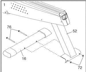
2. Orient the Front Stabilizer (15) as shown. While another person lifts the front of the Frame (1), attach the Front Stabilizer to the Frame with two M10 x 112mm Carriage Bolts (76) and two M10 Nylon Locknuts (72).
