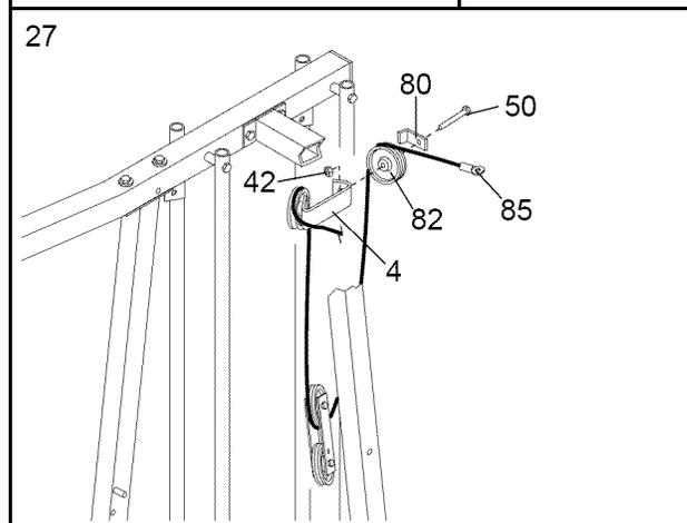
28. **Note: The Left Arm (6) is shown removed for easier part identification.** Slide the other end of the Butterfly Cable (85) onto a 3/8" x 1" Bolt (77). Insert the Bolt through the bracket on the Left Arm (6). Thread a 3/8" Nylon Locknut (42) onto the Bolt, **but do not fully tighten it. Leave just enough room for the Cable to pivot.**
