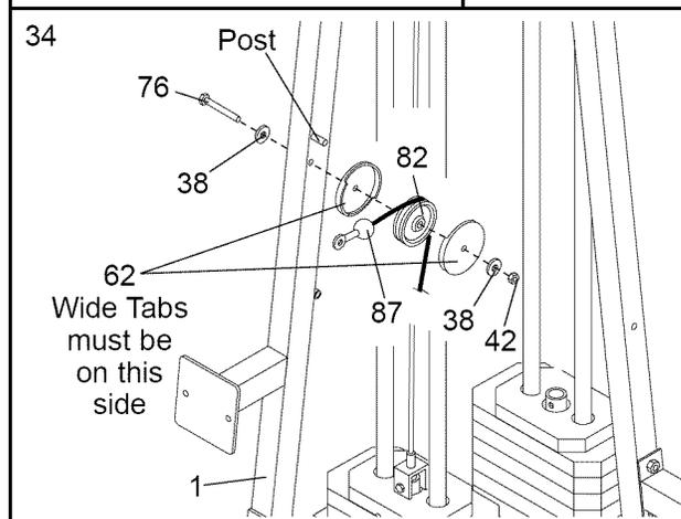
35. Wrap the Rear Cable (87) around a 3 1/2” Pulley (82). Attach the Pulley and two Pulley Covers (62) to the Ab Upright (1) with a 3/8” x 4” Bolt (76), two 3/8” Washers (38) and a 3/8” Nylon Locknut (42). **Do not overtighten the Nylon Locknut; the Pulley should turn easily. Make sure that the Cable is between the Pulley and the post.**
