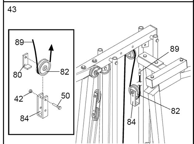
44. Wrap the Low Cable (89) around a 3 1/2" Pulley (82). Attach the Pulley to the Top Frame (2) with a 3/8" x 2" Bolt (50) and a 3/8" Nylon Locknut (42). **The Cable must be routed from the direction shown.**
