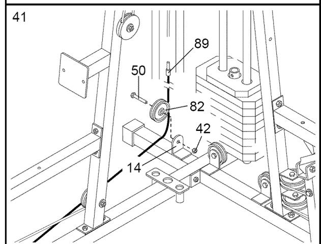
42. Wrap the Low Cable (89) around a 3 1/2" Pulley (82). Attach the Pulley to the indicated bracket on the Top Frame (2) with a 3/8" x 2" Bolt (50) and a 3/8" Nylon Locknut (42). **The Cable must be routed from the direction shown.**
