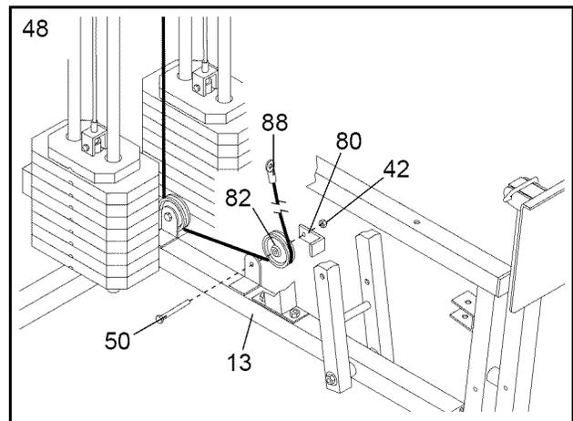
49. Route the Press Cable (88) over the indicated 3 1/2" Pulley (82) attached to the Pulley Plates (31). **The Cable must be routed from the direction shown. Refer to the inset drawing. Be sure that the Cable is between the Cable Trap (80) and the Pulley, and that the Cable Trap is positioned to hold the Cable in place.**
