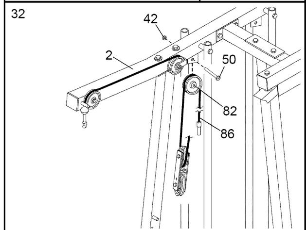
33. Attach the High Cable (86) to a Small “U” Bracket (32) with a 1/4” Nylon Locknut (44) and a 1/4” Washer (37). **Do not completely tighten the Nylon Locknut. It should be threaded onto the end of the Cable so only a couple of threads are showing above the Nylon Locknut, as shown in the inset drawing.**
