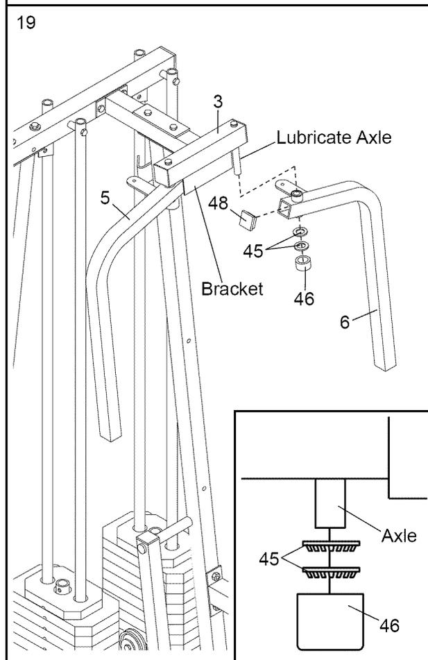
**IMPORTANT NOTE: Before assembling the 1" Retainers (45) used in this step, be sure that you thoroughly understand the step. The Retainers can be assembled only once. If they must be removed, you will need to order new Retainers.**
