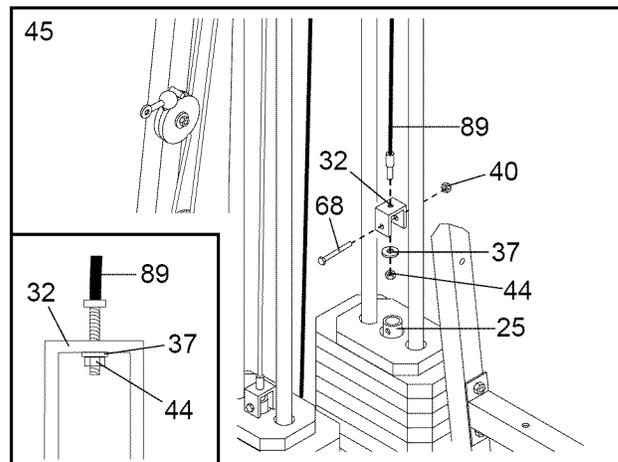
46. **Find the Press Cable (88).** Attach the end of the Press Cable (88) to the Large “U” Bracket (84) with a 1/4” Nylon Locknut (44) and a 1/4” Washer (37). **Do not completely tighten the Nylon Locknut. It should be threaded onto the end of the Cable so only a couple of threads are showing above the Nylon Locknut, as shown in the inset drawing.**
