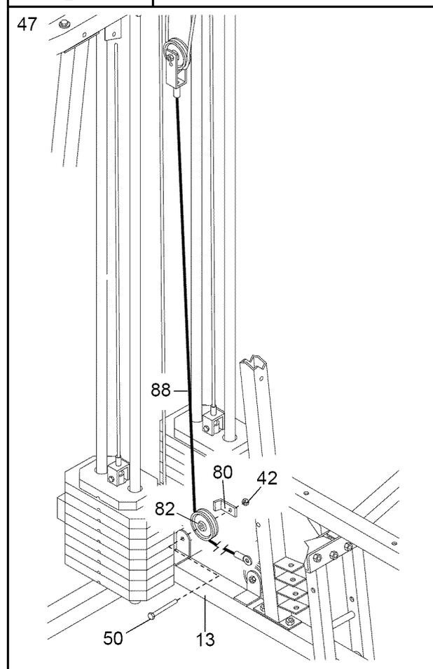
48. **Note: The 3 1/2" Pulley (82) in this step is pre-assembled. It is shown dis-assembled for easier part identification.**
