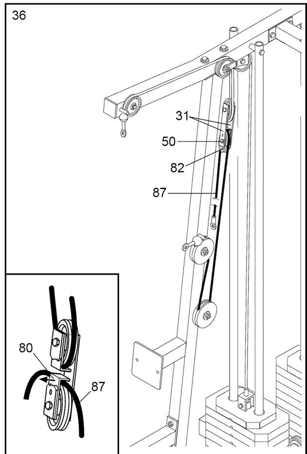
37. Wrap the Rear Cable (87) around a 3 1/2" Pulley (82). Attach the Pulley and a Cable Trap (80) to the Ab Upright (1) with a 3/8" x 3 1/2" Bolt (66), a 3/8" Washer (38) and a 3/8" Jam Nut (43). **Be sure that the Cable and Pulley move smoothly and that the Cable is between the Pulley and the post.**
