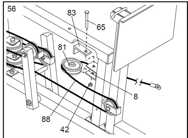
57. **Note: The  $3\ 1/2"$  Pulley (82) used in this step was attached in step 55. It is shown removed for easier part identification.**
