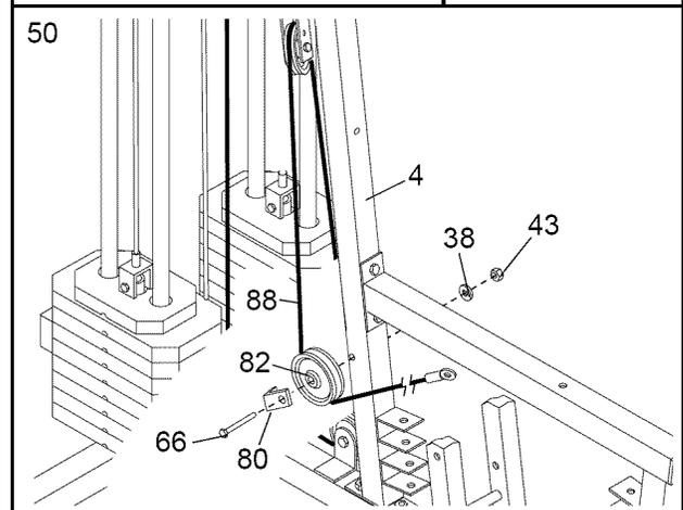
51. Wrap the Press Cable (88) around a 3 1/2" Pulley (82). Attach the Pulley and a Cable Trap (80) to the indicated hole in the Press Frame (12) with a 3/8" x 3 1/2" Bolt (66), a 3/8" Washer (38) and a 3/8" Nylon Locknut (42). **Be sure that the Cable Trap is turned to hold the Cable in place.**
