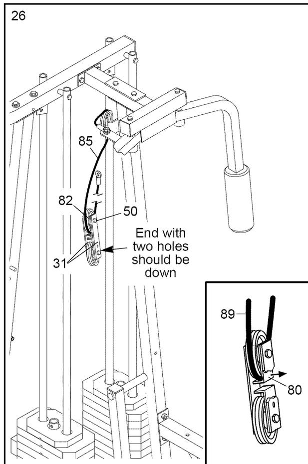
27. Wrap the Butterfly Cable (85) around a 3 1/2" Pulley (82) as shown. Attach the Pulley and a Cable Trap (80) to the other side of the bracket on the Leg Press Upright (4) with a 3/8" x 2" Bolt (50) and a 3/8" Nylon Locknut (42). **The Cable Trap must be oriented as shown and be positioned to hold the Cable in the groove of the Pulley.**
