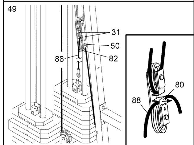
50. Wrap the Press Cable (88) around a 3 1/2" Pulley (82). Attach the Pulley and a Cable Trap (80) to the Leg Press Upright (4) with a 3/8" x 3 1/2" Bolt (66), a 3/8" Washer (38) and a 3/8" Nylon Jam Nut (43). **Be sure that the Cable Trap is turned to hold the Cable in place.**
