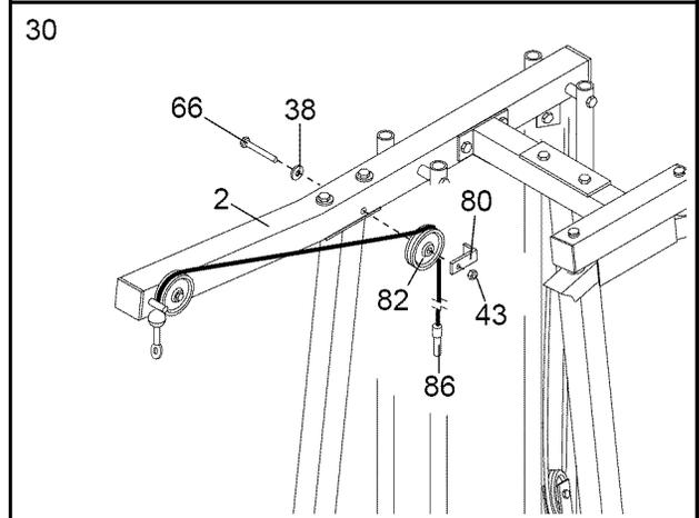
31. **Locate the remaining pre-assembled pair of Pulley Plates (31) and 3 1/2" Pulleys (82).**
