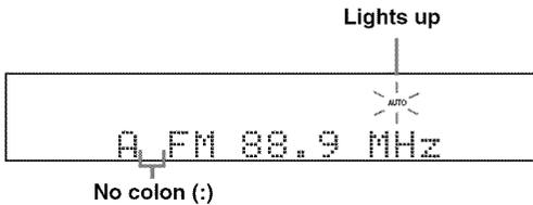
If a colon (:) appears in the front panel display, automatic tuning is not possible. Press **Ⓢ** **PRESET/TUNING** to turn the colon (:) off.
