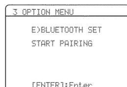
Use this feature to start pairing the connected Yamaha Bluetooth adapter (such as YBA-10, sold separately) with your Bluetooth component. For details about the pairing, refer to “Pairing the Bluetooth™ adapter and your Bluetooth component” on page 59.
