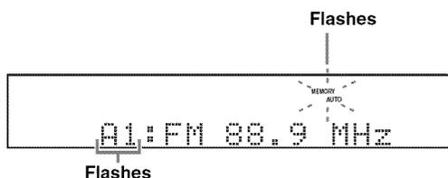
When automatic preset tuning is completed, the front panel display shows the frequency of the last preset station.
