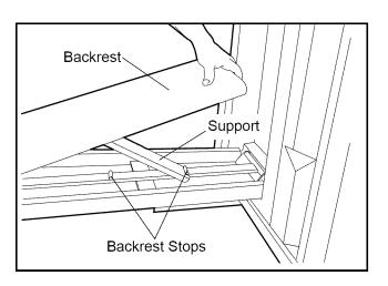
To adjust the backrest to the level position, first raise the backrest slightly. Pivot the end of the support in the direction shown by the arrow. Lower the backrest onto the bench frame.
