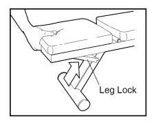
Next, raise the bench to the vertical position and hold it in place. Using your right hand, slide the bench knob to the left as far as possible. Make sure that the knob is moved all of the way to the "treadmill" position. Refer to the inset drawing. Make sure that the lock pin is inserted
