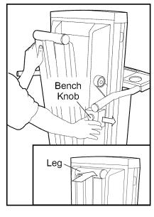
on the leg while you slide the knob to the "bench" position (refer to the inset drawing above).
