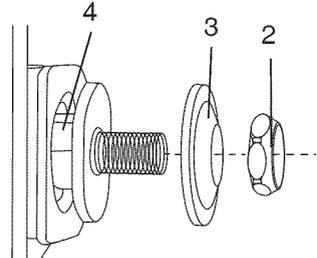
3. Place the blade onto the arbor (4) with the blade teeth pointing forward to the front of the saw. (Fig. N)
