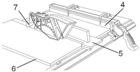
8. Continue pushing the workpiece (6) with the push stick (3-Fig. QQ) or push block until it passes through the blade guard and clears the rear of the table. (Fig. RR)
