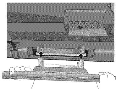
3 Drive Phillips pan screws in the 2 threaded holes with a screwdriver tightly.
