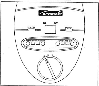
POWER CONTROL SWITCH and INDICATOR LIGHT - This switch will turn the air cleaner ON or OFF and has three speed selections: III (super), II (high) and I (low).
