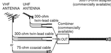
• Connect the antenna cable to the TV using one of the methods in the illustration as shown (1, 2, 3 or 4).
