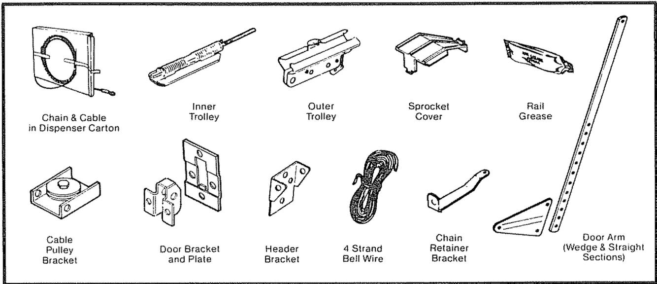
SEPARATE ALL HARDWARE FOR ASSEMBLY AND INSTALLATION PROCEDURES AS SHOWN BELOW.
