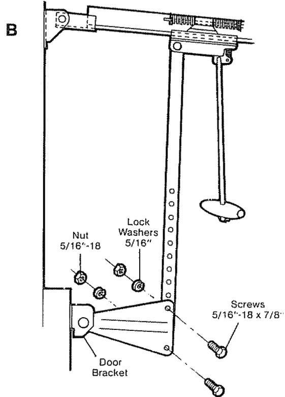
Bring the door arm sections together. Find a pair of holes that line up and join sections as shown (B).
