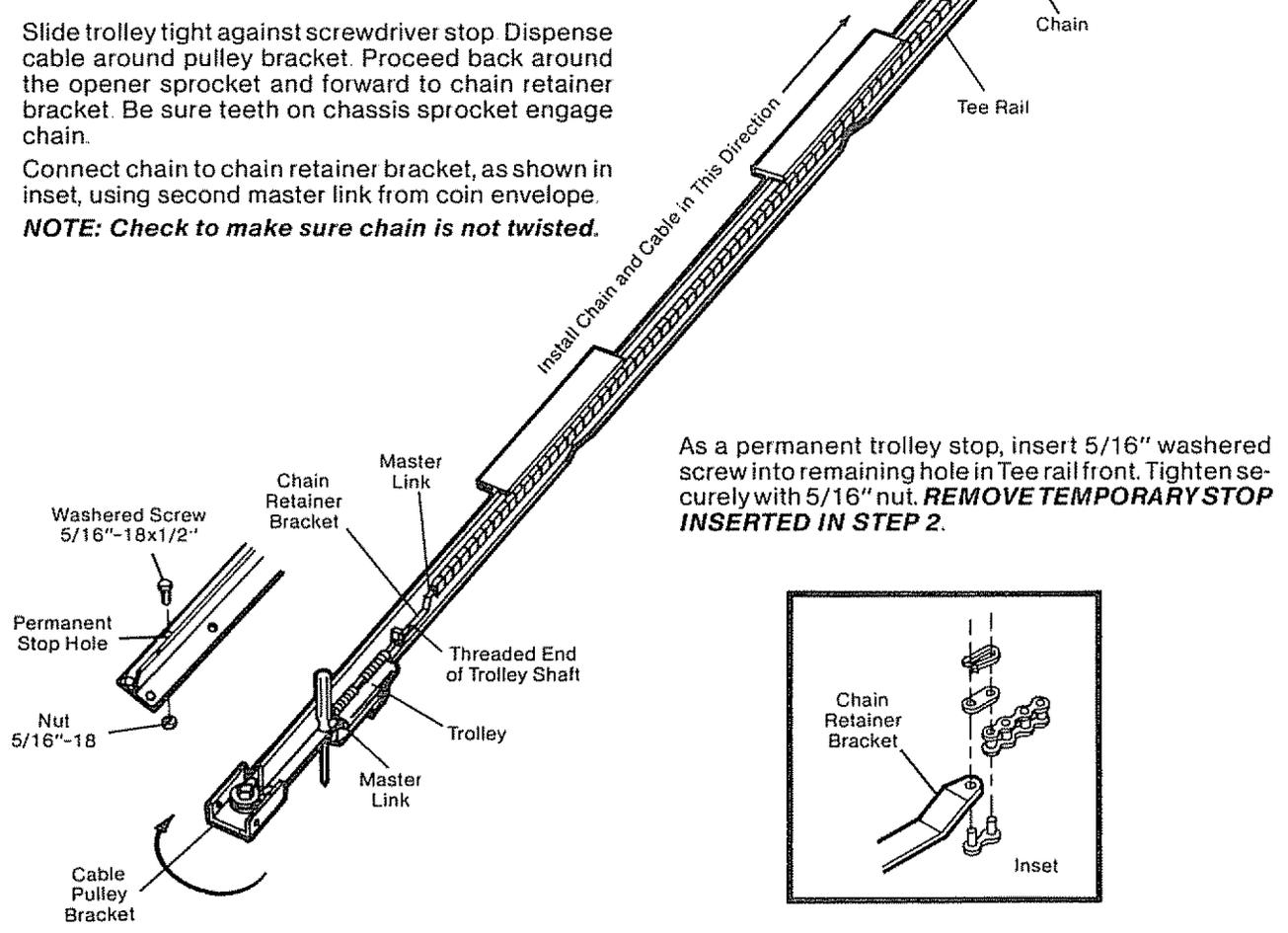
As a permanent trolley stop, insert 5/16" washered screw into remaining hole in Tee rail front. Tighten securely with 5/16" nut. **REMOVE TEMPORARY STOP INSERTED IN STEP 2.**
