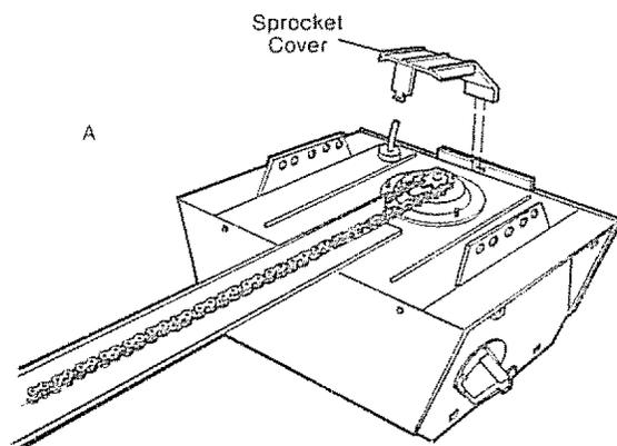
**PROCEDURE:** Attach sprocket cover to chassis as shown in Illustrations (A) and (B). Insert back tab in chassis slot. Then bend cover forward and insert front tab in slot provided on mounting plate.
