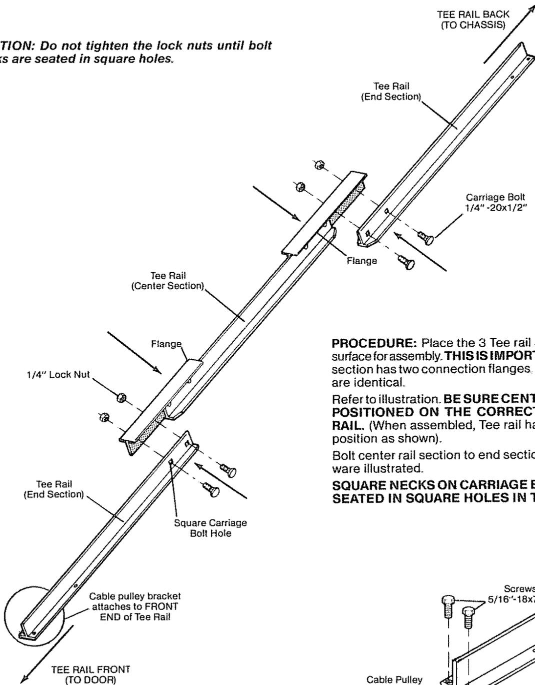
**PROCEDURE:** Place the 3 Tee rail sections on a flat surface for assembly. **THIS IS IMPORTANT.** The center section has two connection flanges. The end sections are identical.
