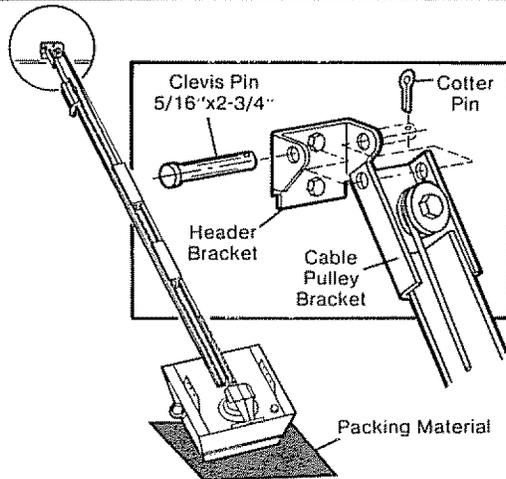
**PROCEDURE:** Position opener chassis on garage floor below door and header brackets. Use packing material base to protect cover. **NOTE:** To enable Tee rail to clear sectional door springs, it may be necessary to lift the chassis onto a temporary support.
