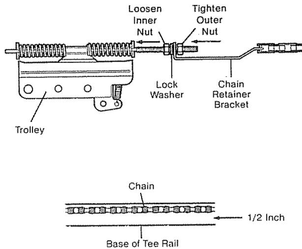
**PROCEDURE:** Connect chain and cable to threaded shaft of trolley in the order illustrated: inner nut, lock-washer, chain retainer bracket and outer nut.
