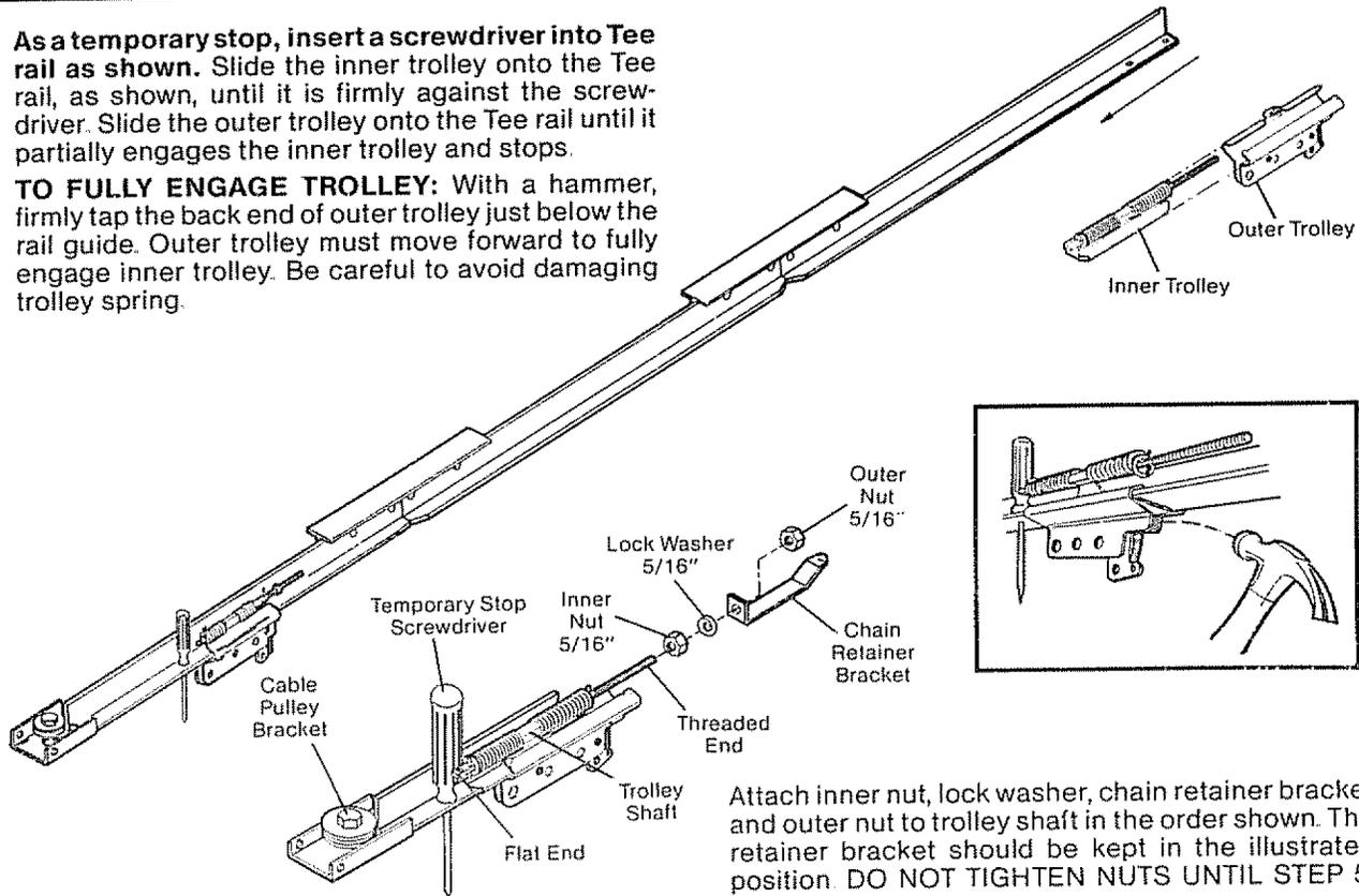
Attach inner nut, lock washer, chain retainer bracket and outer nut to trolley shaft in the order shown. The retainer bracket should be kept in the illustrated position **DO NOT TIGHTEN NUTS UNTIL STEP 5, PAGE 9**
