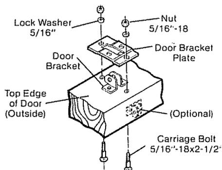
**NOTE:** Door bracket may be installed on face of door if required for your installation. (Refer to dotted line drawing). **HOWEVER,** drill 3/16" pilot holes and substitute 5/16" x 1-1/2" lag screws (not supplied) to fasten bracket to door.
