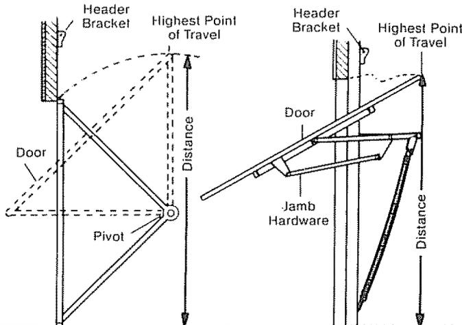
Locate height for header bracket by opening door to highest point of travel as shown. Measure distance from top of door to floor. Subtract actual height of door. Add 8" to the remainder. See example below.
