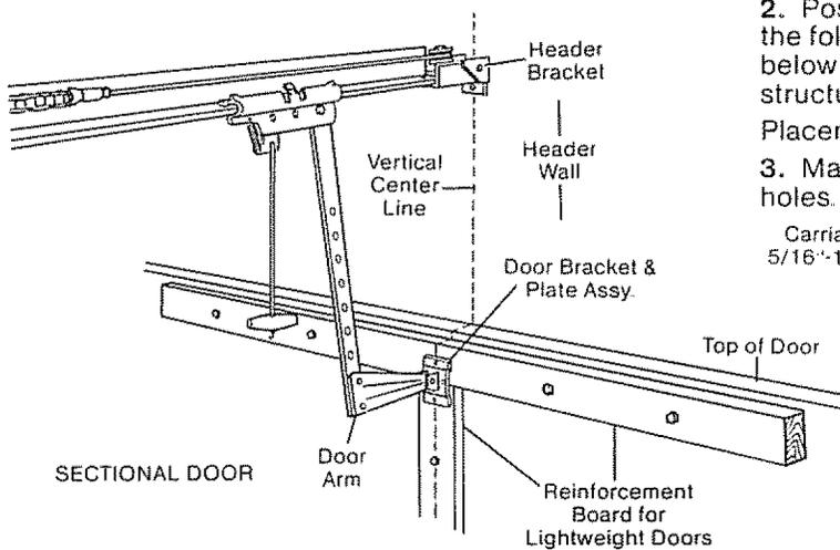
1. Assemble door bracket and plate as shown. Center bracket on vertical guideline (or up to one foot left or right of center if necessary).
