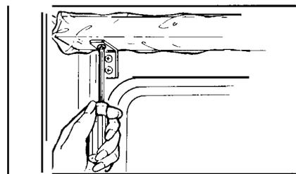
Remove the two mounting screws as shown and pull the top toward you to remove it from the dishwasher.
