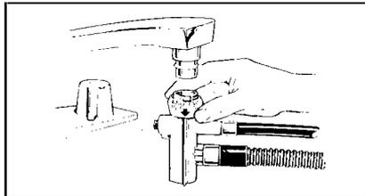
2. Attach the Unicouple connector to the faucet adapter by depressing collar at the top of the connector." When Unicouple is all the way up onto the adapter, release the collar. It will then snap into position to lock the Unicouple in place.
