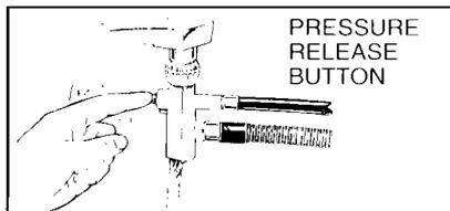
The Faucet-Flo nozzle is part of the Unicouple connector." Operate the nozzle by depressing the pressure release button on the front of the Unicouple connector. YOU will find the Faucet-Flo nozzle useful for several reasons. For example:
