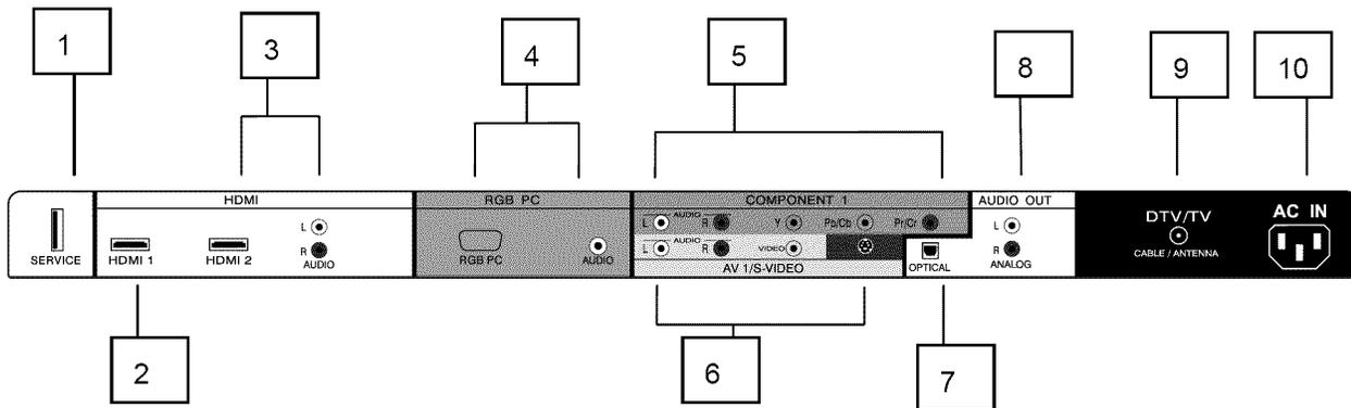
1. **SERVICE** – This custom communication port is for factory service only. **Use of this input for any purpose other than factory authorized service will void the manufacturer’s warranty of this equipment.**
