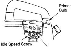
Mixture Screw with Limiter Cap
