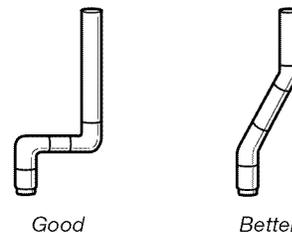
4. Use clamps to seal all joints. Do not use duct tape, screws or other fastening devices that extend into the interior of the vent to secure vent.
