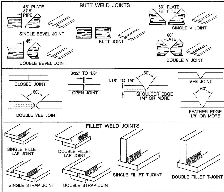
**Figure 3. Types of Weld Joints**
