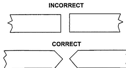
Figure 2. Workpiece Preparation
