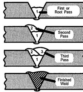
Figure 13. Triple Pass V Butt Joint
