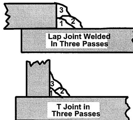
Figure 14. Triple Pass Lap and T Weld Joint
