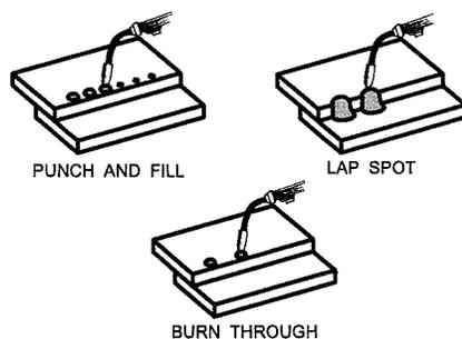
**Figure 15.** Spot Weld Methods
