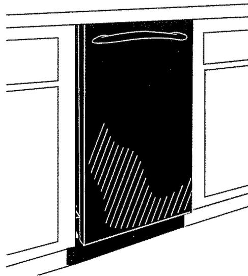
**IMPORTANT** – The dishwasher **MUST** be installed to allow for future removal from the enclosure if service is required.
