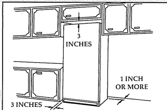
Allow three inches of air space on all sides of the freezer.
