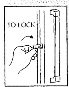
Key pops out for security – store in safe place. To lock or unlock the freezer you must push the key in the lock while turning. The lock is spring loaded so the key cannot be left in the lock.
