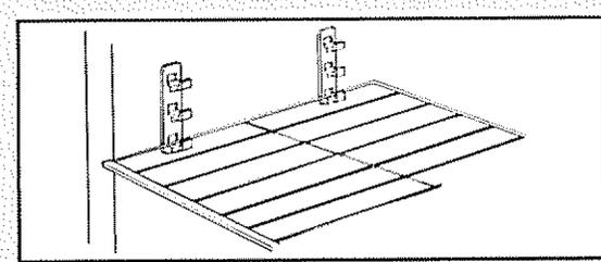
Three position adjustable shelf can be moved to any one of three positions for larger or smaller packages.
