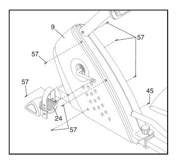
With the left shield removed, locate the Reed Switch (43). Turn the Crank (31) until the Magnet (38) is aligned with the Reed Switch. Next, loosen, but do not remove, the indicated M4 x 16mm Screw (57). Slide the Reed Switch slightly closer to or away from the Magnet, and then retighten the Screw. Turn the Crank for a moment. Repeat until the console displays correct feedback. When the Reed Switch is correctly adjusted, reattach the left shield and the left pedal.
