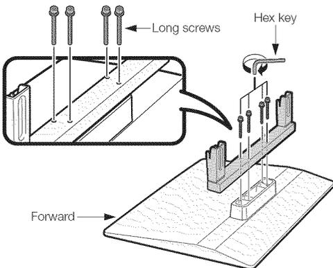
3 ① Insert the stand into the openings on the bottom of the TV.
