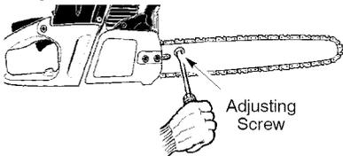
4. Using a screwdriver, roll chain around guide bar to ensure all links are in bar groove.
