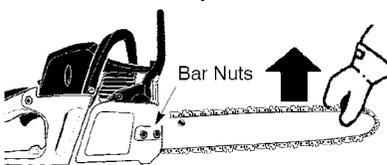
7. Use a screwdriver to move chain around guide bar.
