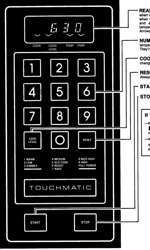
**READOUT DISPLAY** - Remains blank when oven is not in use. Shows remaining time when cooking by time. Shows set temperature and actual temperature when cooking to temperature.
