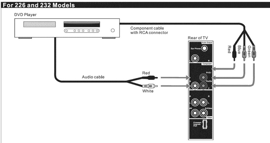
**Note:** The Y, Pb and Pr jacks do not provide audio, so audio cables must be connected to provide sound.
