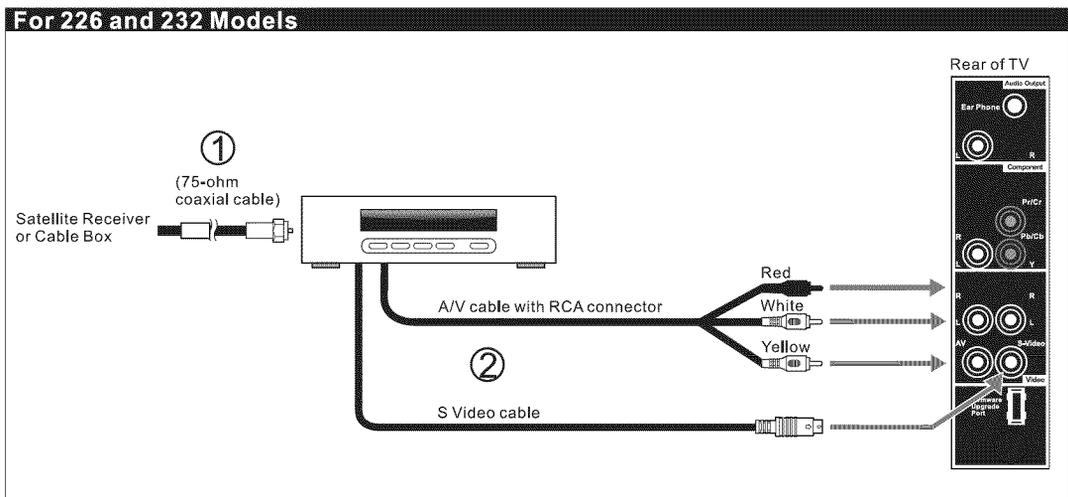
**Note:** When you connect video equipment to both the same Video and S-Video input jacks, display will automatically select S Video first.
