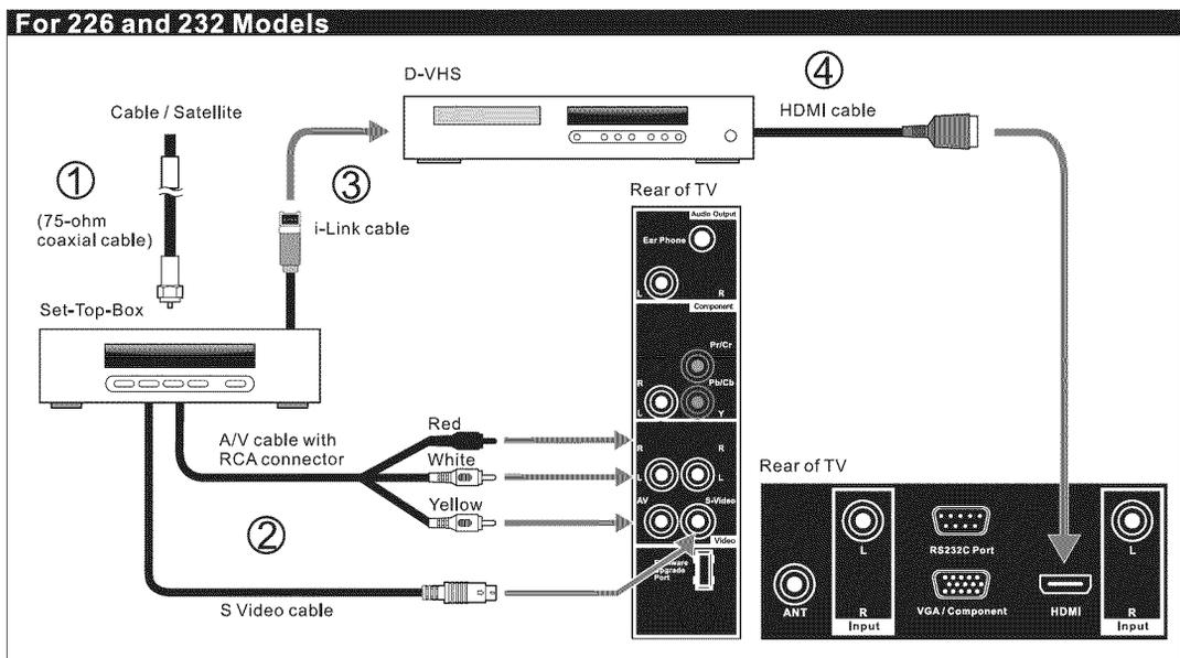
**Note:** HDCP is a copy protected digital connection that receives analog or digital video and audio signals from equipment with a HDMI output that features the HDCP function. HDMI allows the transfer of digital uncompressed data to the TV. This connection is superior when compared to the Component, S Video or AV (composite) connections.
