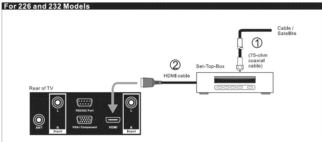
**Note:** HDCP is a copy protected digital connection that receives analog or digital video and audio signals from equipment with a HDMI output that features the HDCP function. HDMI allows the transfer of digital uncompressed data to the TV. This connection is superior when compared to the Component, S Video or AV (composite) connections.
