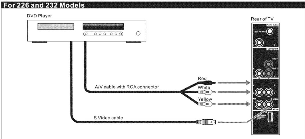
**Note:** When you connect video equipment to both the same Video and S-Video input jacks, the display will automatically select S-Video first.
