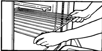
1. Position the rack(s) properly **before** turning on the oven. To **change rack position**, lift rack at front and pull out.
