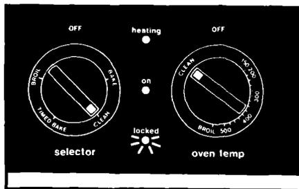
5. The "locked" Signal Light comes on when the oven temperature exceeds normal baking temperatures. The Lock Lever must not be moved and the door can't be opened when the "locked" Signal Light is on.
