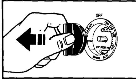
1. Pull the Oven Temperature Control Knob straight off.
