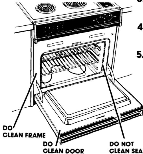
**DO NOT clean the fiberglass seal. DO NOT move it or bend it. Poor cleaning and poor baking will result.**
