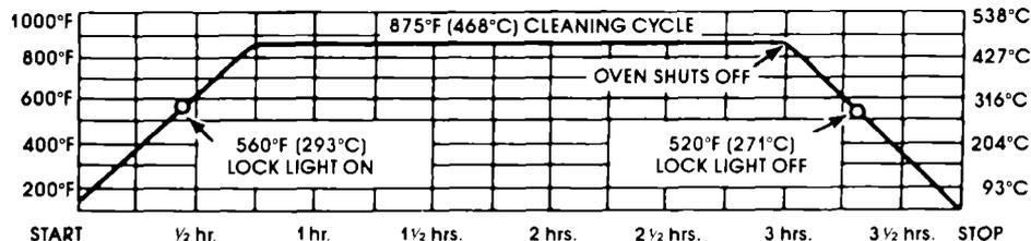
Notice that the heating stops when the 3-hour setting is up, but that it takes longer for the oven to cool down enough to unlock.
