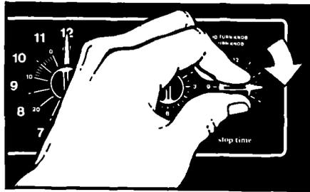
3. Push in and turn the Stop Time Knob **clockwise** 2 or 3 hours.
