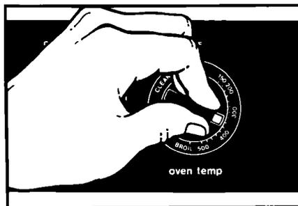
3. Set the Oven Temperature Control to the baking temperature you want. The "heating" Signal Light will come on. The oven is pre-heated when the "heating" Signal Light first goes off.
