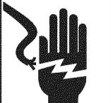
**FOR PERSONAL SAFETY:** Remove house fuse or open circuit breaker before beginning installation. Do not use an extension cord or adapter plug with this appliance.
