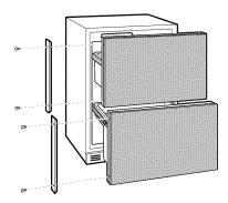
• Place the brushed decorative covers over the side trim to hide the screw heads. Ensure side trim is aligned top to bottom and front to back. Snap into place.
