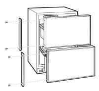
• Custom handles of your choice, supplied by your cabinet maker, must be installed onto the overlay panels before they are slid into the trims. Countersink all screws into the backer panels. Screws cannot protrude from the backer panels.
