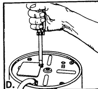
D. Once the disposer is off, turn it upside down and remove the electrical plate.
