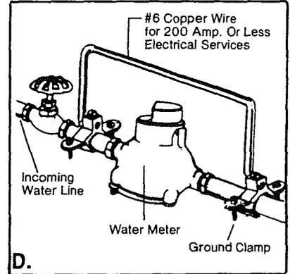
**WARNING:** IF NOT PROPERLY GROUNDED, a hazard of electrical shock may exist. DO NOT reconnect electrical power at main service panel until proper ground is installed. For your safety, DO NOT ground to a gas supply pipe.
