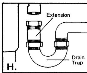
**TUBE TOO SHORT?** If the discharge tube doesn't reach your drain trap outlet, measure the difference. Then buy a drain extension tube.
