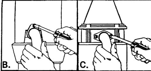
Turn the disposer around to attach the discharge tube. Some models use a rubber washer that must be assembled to the discharge tube before putting the metal flange over the discharge tube, see 'D'. Secure metal flange using the edge tab on the flange and screw. On other models, put the rubber washer in the discharge tube opening. Slip the metal flange over the discharge tube. Using the screw(s) provided, attach the flange to disposer, see 'E'.
