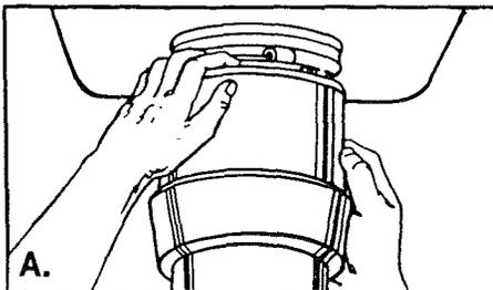
Lift the disposer and place it so the disposer's three mounting lugs are lined up *under* the three sink mounting assembly screws.
