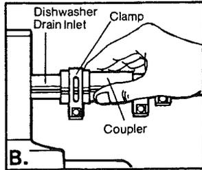
Slide large end of rubber coupler, from dishwasher drain connection kit, over the inlet tube of the disposer. Fasten the coupler to disposer with the clamp provided.
