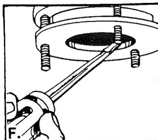
F. Loosen screws and remove old mounting ring and back-up ring. You may need a hammer to loosen assembly parts.
