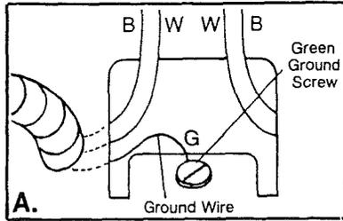
If the cable leading to the disposer does not have a ground wire, use a copper wire that is no smaller than the other wire in your cable. Attach one end of the wire to the green ground screw on the disposer.
