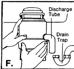
Turn the disposer so that the discharge tube lines up with your drain trap. Slip the drain trap over the discharge tube.
