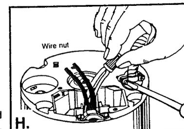
Install the cable connector. Then loosen the connector screw(s). Work the cable from the on-off switch through the connector so that the leads are in the electrical wiring area in the disposer base.
