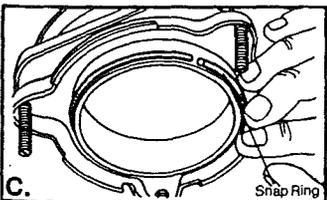
Now, push the fiber gasket, metal back-up ring and the mounting ring further up on the sink sleeve. Slide the snap ring onto the sink sleeve until it pops into place in the groove on the sleeve.
