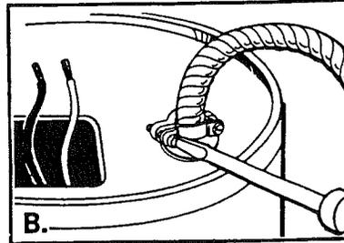
Now, tighten the connector clamp screw(s) to hold the cable in place.
