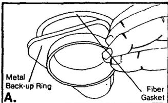
First, working from under the sink, slip the fiber gasket and next the metal back-up ring (flat side up) up and over the sink sleeve.
