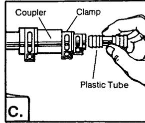
Insert one end of the plastic tube into the coupler and fasten with  $\frac{1}{8}$  inch clamp.
