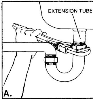
A. Use a pipe wrench to loosen the nut at the top of the drain trap.
