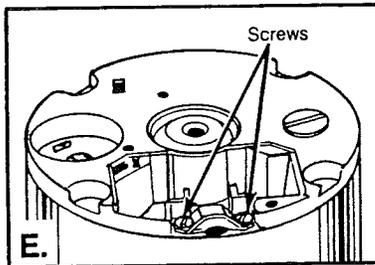
If you are using the built-in cable clamp **loosen** the two screws until cable will freely enter under the clamp.
