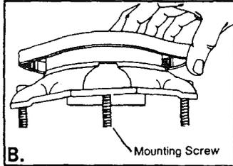
Then loosen the screws on the mounting assembly until they are just level with the surface of the mounting ring.
