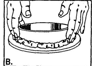
Apply this roll under the rim of the sink sleeve.
