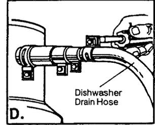
Slip the remaining clamp (the one you purchased) over the dishwasher drain hose and back two or three inches. Now, slip the drain hose over the plastic tube, slide the clamp into place and tighten.
