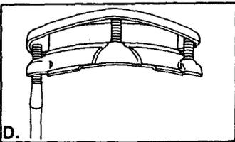
Tighten the three mounting screws with your screwdriver until the whole mounting assembly is seated evenly and tightly against the sink.
