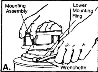
First, remove the mounting assembly from the lower mounting ring. Holding the mounting assembly with one hand, insert your wrenchette or screwdriver into one of the lugs of the lower mounting ring and turn it to the left (counterclockwise) with your other hand.
