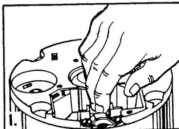
Finally, place the connected wires back in the compartment. Replace electrical plate.
