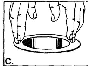
Then, place the sink sleeve into the sink drain hole and push down gently but firmly to make sure it sits evenly in the putty.
