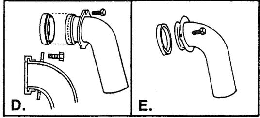
In D, install the discharge tube gasket onto the discharge tube. Gasket must be installed as shown to assure a leak-proof installation. In E, install discharge tube gasket into disposer discharge outlet. Gasket will be held in place by the discharge tube flange.
