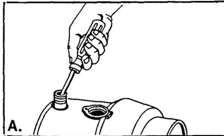
Lay the disposer on its side and put the tip of your screwdriver into the dishwasher drain hole opening at an angle.
