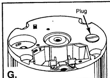
If you are using "Greenfield" Cable then the plug must be removed.
