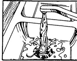
Run water through the disposer. Then, place the stopper in the sink sleeve in the seal position. Fill the sink with water.
