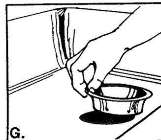
G. Finally, remove the old sink sleeve by pushing it up through the sink hole.
