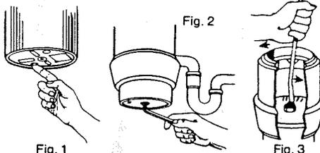
A pry bar or tool should be inserted through the sink opening into the disposer. The end then must be placed alongside the grinding protrusion near the outside edge of the grinding disc. Be sure to place the pry tool on the proper side of the protrusion so when pressure is applied the grinding disc will move in the proper direction to unjam the disposer. (see Fig. 3). Do not drop or hammer on pry bar.
