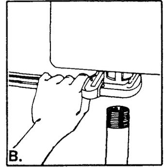
B. Next, remove the nut at the top of the sink strainer and remove the extension tube.
