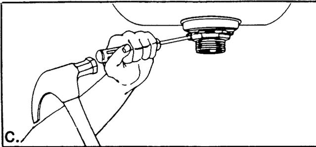
C. Now, remove the large nut at the base of the sink strainer by placing the tip of your screwdriver on the edge of the nut. (There are usually ridges to hold your screwdriver.) Then strike the head of the screwdriver with a hammer in a counterclockwise direction.
