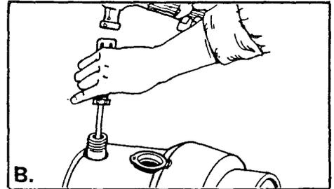
Tap the end of the screwdriver with a hammer until the molded plug pops out. **Make sure you take the loose plug out of your disposer.**
