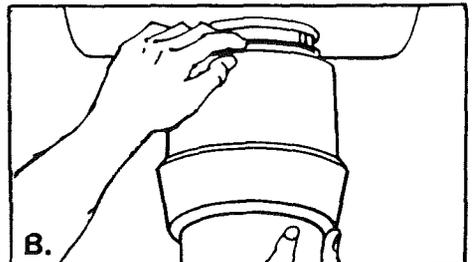
Then, while holding the disposer in place, turn mounting ring with the lugs to the right until all *three* ears are engaged on the mounting assembly. The disposer will now hang by itself. You will lock this ring later, after the plumbing connections are made.
