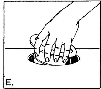
E. Now, push the strainer up through the sink hole and remove it.
