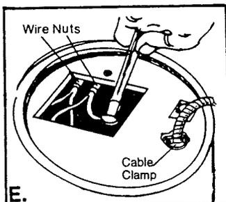
E. Now, use a screwdriver to remove ground wire. Remove the wire nuts from the power wires. Separate the disposer power wires from the cable wires. Loosen the screw(s) on the cable clamp and remove the cable from the disposer.
