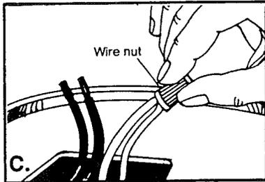
Connect the two power wires to the cable wires, making sure you connect **white to white** and **black to black**. Secure the wires with wire nuts by twisting them to the right (clockwise).
