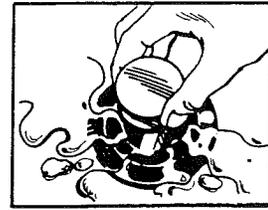
Finally, remove the stopper and let the water drain. Check for leaks at all plumbing connections and at the top of the disposer and correct, if you need to.
