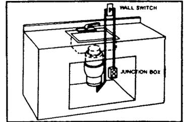
It will be necessary to install a 20 amp. wall switch above the countertop and a junction box under the sink as illustrated.
