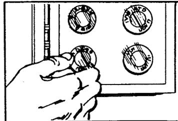
First, remove the fuse or turn off the circuit breaker on the circuit you plan to use for your disposer. Use a separate 15 or 20 amp., 115 volt circuit for the disposer.
