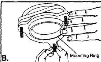
Hold the fiber gasket and metal back-up ring in place with one hand and place the mounting ring with its three screws onto the sink sleeve.
