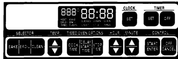
If you have electronic controls: Push the "BAKE" pad and "350°" will appear in the display. Press the "START/ENTER" pad and "Lo°", "HEAT" and "BAKE" will appear in the display. **The oven burner should light in 50 to 60 seconds. This delay is normal.** The oven safety valve requires a certain time before it will open and allow gas to flow.
