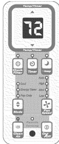
Note: Tap or hold either up (▲) or down (▼) button until the desired temperature is seen on the display. This temperature will be automatically maintained anywhere between 60°F (16°C) and 90°F (32°C). If you want the display to read the actual room temperature. See "To Operate on Fan Only" section on Page 7.
