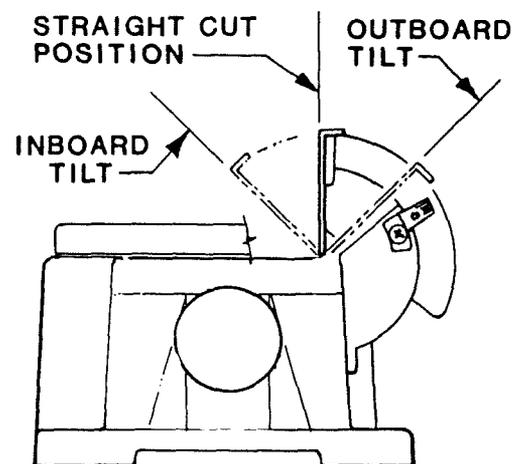
**CHAMFERING** is removing only the corner of the edge of a board. Normally a chamfer is made with one cut; therefore, a cut deeper than  $\frac{1}{16}$ " may be made.
