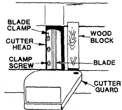
2. Locate the slot in the cutter head shaft through the small hole in the backside of the machine directly above the vacuum port. Rotate the cutter head with a screwdriver until one of the blades is at its highest position.
