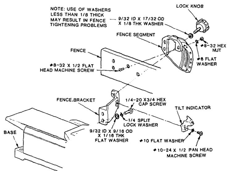
5. Place square against face of fence and table surface. Bring fence square to table and tighten lock knobs.
