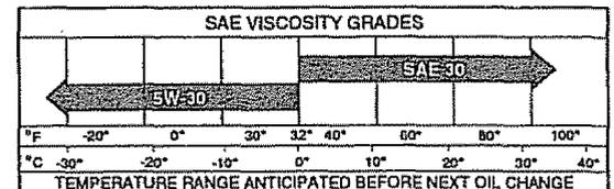
**NOTE:** Although multi-viscosity oils (5W30, 10W30 etc.) improve starting in cold weather, these multi-viscosity oils will result in increased oil consumption when used above 32°F. Check your engine oil level more frequently to avoid possible engine damage from running low on oil.
