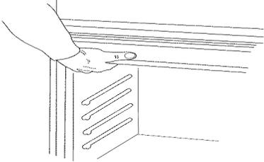
2. Push against seal area of front frame to push oven into cabinet until shipping feet almost contact cabinet.
