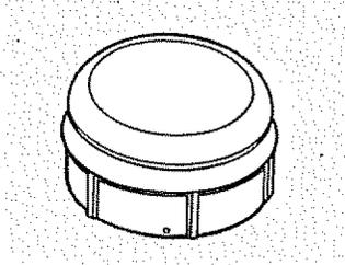
The **agitator cap** fits into the top of the agitator. If it accidentally comes off, simply put it back on.
